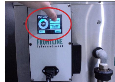
**Step 1:** Push and hold down the Dispose button.
