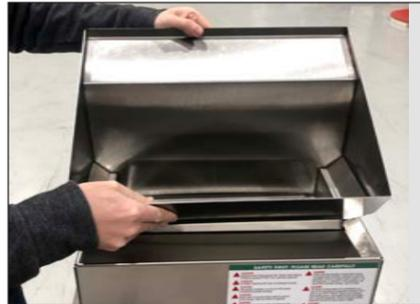
**Step 1:** Remove Grill Grease Caddy chute and basket and set to the right of the Caddy.
