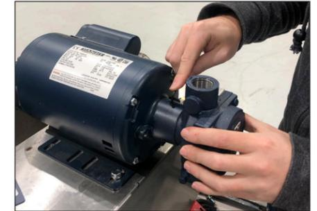
**Step 12:** Using an Allen wrench, loosen (don't remove) the three pins holding the pump head to the motor.
