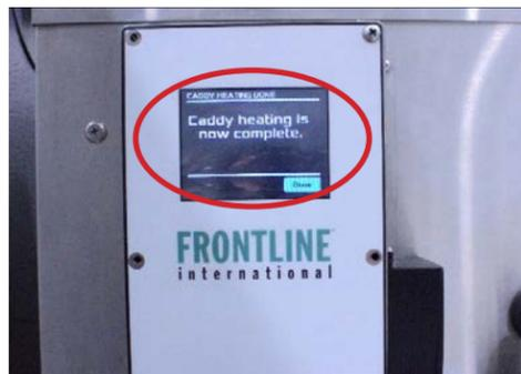
**Step 3:** After the heating process time has passed, a message will appear on the control panel display.
