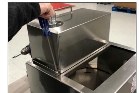
**Step 18:** Resecure the motor housing back to the caddy using the four screws. ■
